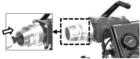
11. Put antifreeze (undiluted 50 ml/(0.013 gal(US))) into the strainer guide.
