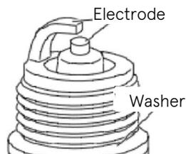
If necessary, adjust the gap to the specification.
