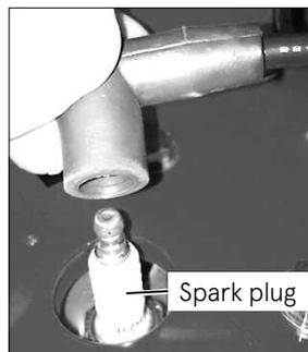
2. Use a wire brush or spark plug cleaner to clean the electrode of the spark plug.
