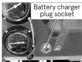
Be sure to charge the battery after each operation.
